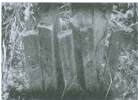
Treated and untreated strips buried half around a termite infested fence post
